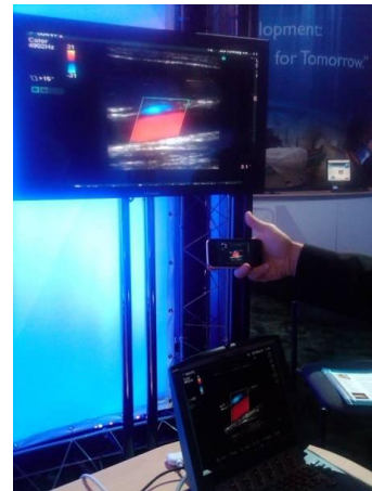
SonicEye® Finger-mounted Ultrasound Probe (left) And iPhone® application capability (right)
