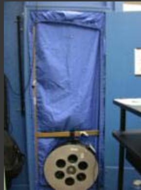
Air tightness testing w/ blower door
