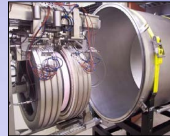
NIST's 0.5 meter Guarded Hot Plate Capable of Providing Measurements of Thermal Insulation from 90 to 900 K
